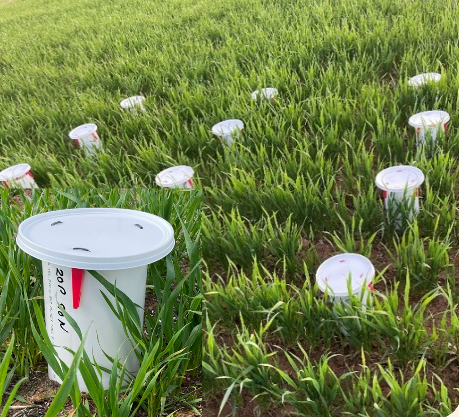
Figure 2. Setup for ammonia measurement in the field.
